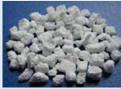
Porous blocks (10mm cubes with 200 \mu m porosity )
