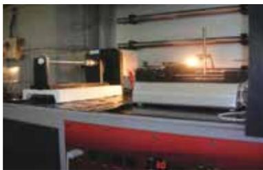
Electrospinning set up for preparing scaffolds
