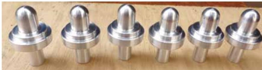
10. Completed the machining of thermowell and thermometer fixture to MPL
