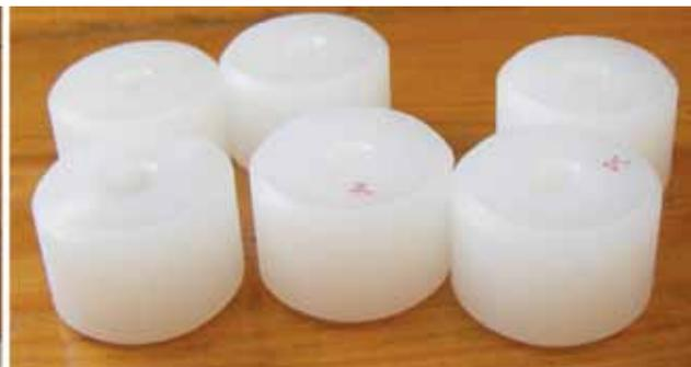
6. Completed the machining of vascular graft coating fixture components to DTL.
