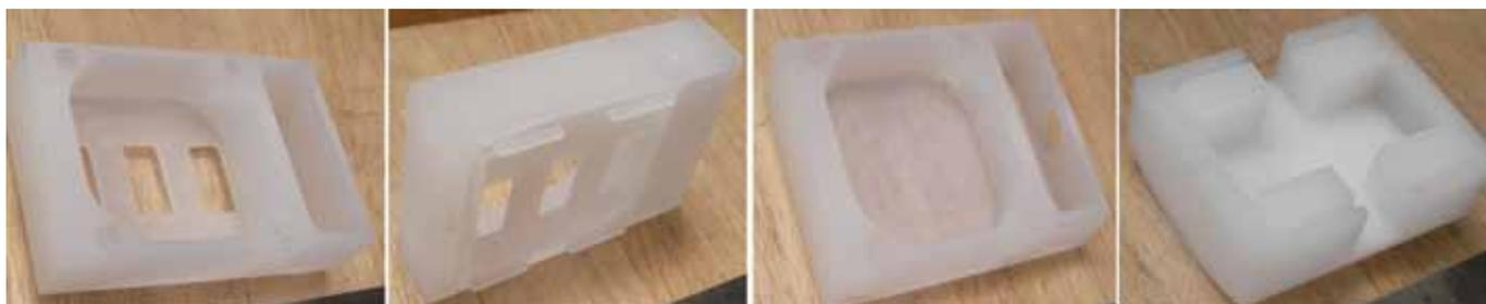
2. Completed the machining of 3 sets of Electromagnetic Flow meter components (Polypropylene- casing, cover and bottom part) to MPL
