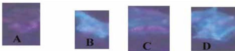
Polymer strips embedded with Cdots and glucose binding ligands. (A) Polymer as such, (B) Polymer and fluorophore (see the blue colour), (C) Polymer, fluorophore and glucose binding molecule (It is clear that fluorescence is significantly quenched by the glucose binding molecule), (D) Polymer, fluorophore, glucose binding ligand and glucose (see the blue colour Quenched fluorescence is revived in the presence of glucose)
