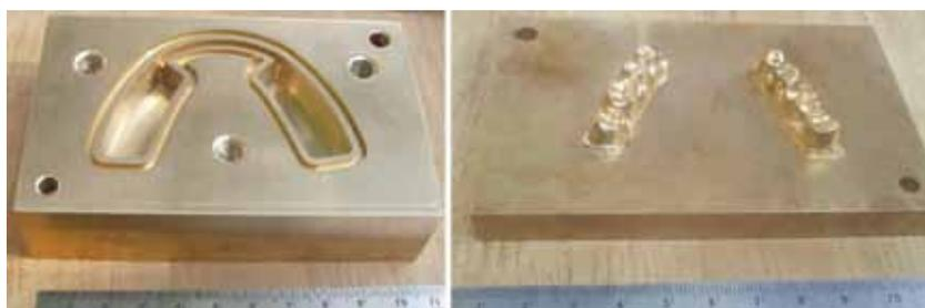
3. Completed the machining of Mandibular Advancement Device mould Core & Cavity to DTL
