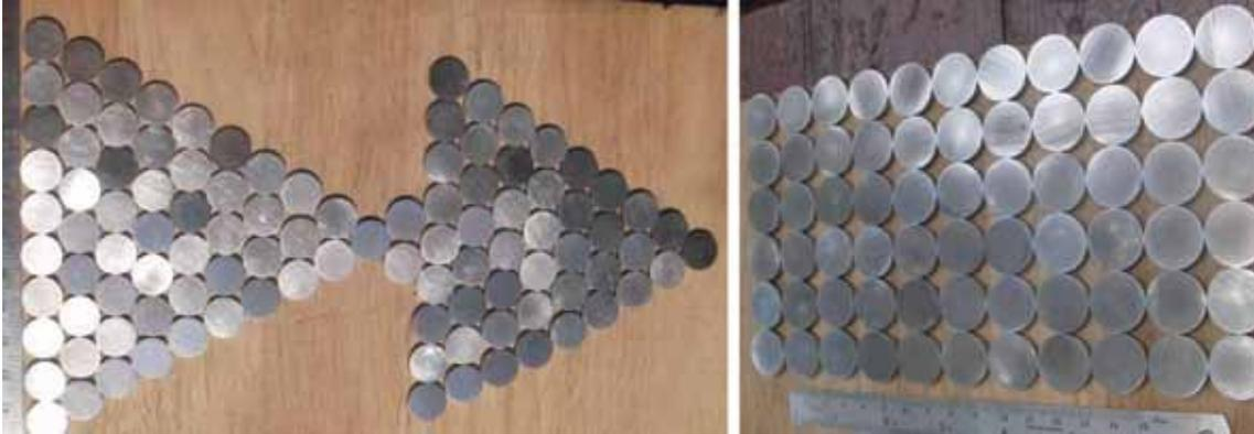
7. Completed the machining of different size blanks for testing the coating to CCF lab.
