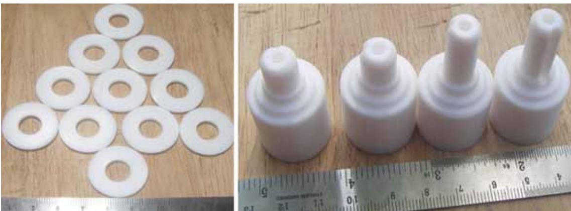
8. Completed the machining of different Teflon moulds, sample preparation rings and Teflon plug to TEM, TIC and MPL lab.
