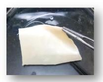
The technical know how for the process of manufacture of glutaraldehyde cross-linked pericardium was developed. The cross-linked pericardium fabricated by this process can be used as a cardiovascular patch or for application in right ventricular outflow tract reconstruction.
