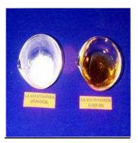
Glass ionomer cement are dental restoratives used for core build up, luting and restorative applications. It is used for prevention of dental caries. The material has good adhesive property with the tooth and hence it act as dental sealant.
