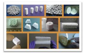
Hydroxyapatite derived materials are used as synthetic bioactive materials for orthopaedic applications due to their molecular structural and compositional similarity with the mineral part of the bone. Porous granule form of hydroxyaptite is a general purpose synthetic bone graft material.
