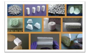
Hydroxyapatite derived materials are used as synthetic bioactive materials for orthopaedic applications due to their molecular structural and compositional similarity with the mineral part of the bone. Porous granule form of hydroxyaptite is a general purpose synthetic bone graft material.
