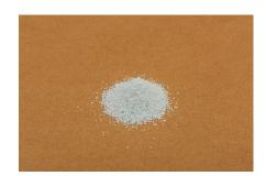
Calcium Phospho-silicate Composite (denoted as HA-BG, indicating hydroxyapatite and bioactive glass composite) is a bioactive ceramic material. This contains a combination of calcium silicate and calcium phosphates phases, including hydroxyapatite. The fine granules (less than 1 mm size grade) are useful for the defects in the alveolar, mandibular or maxillary bone. It be helpful for healing periodontal and furcal defects (arising out of periodontitis), periapical cysts and
