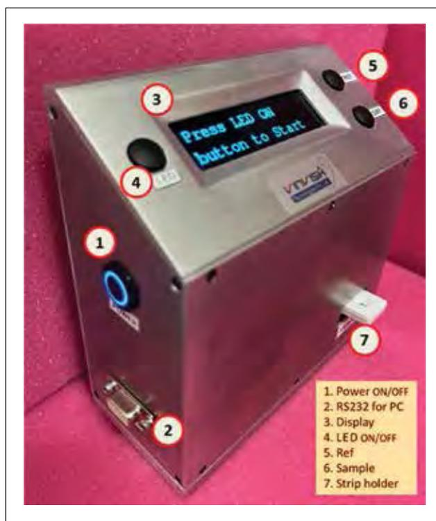
Figure 26: Instrument for measuring NT-proBNP
