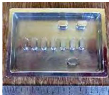
*Mould for developing PDMS*
