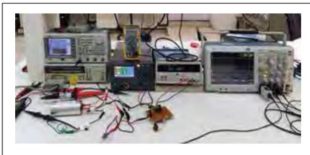
Figure 32: Experimental setup for the evaluation of charging circuit
