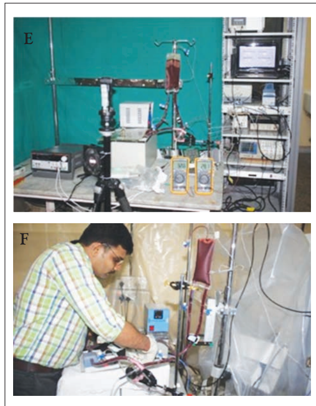
Figure 28. (A) Chitra paracorporeal Left Ventricular Assist Device (pLVAD), (B) pLVAD with controller, battery pack, and charging unit, (C,D) Training on device fabrication and evaluation to industrial partner (E,F) In vitro evaluation of LVAD for estimation of haemolysis
