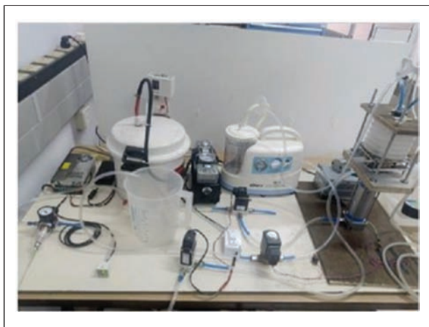
Figure 26. Validation setup for reverse suction and suction arrester device
