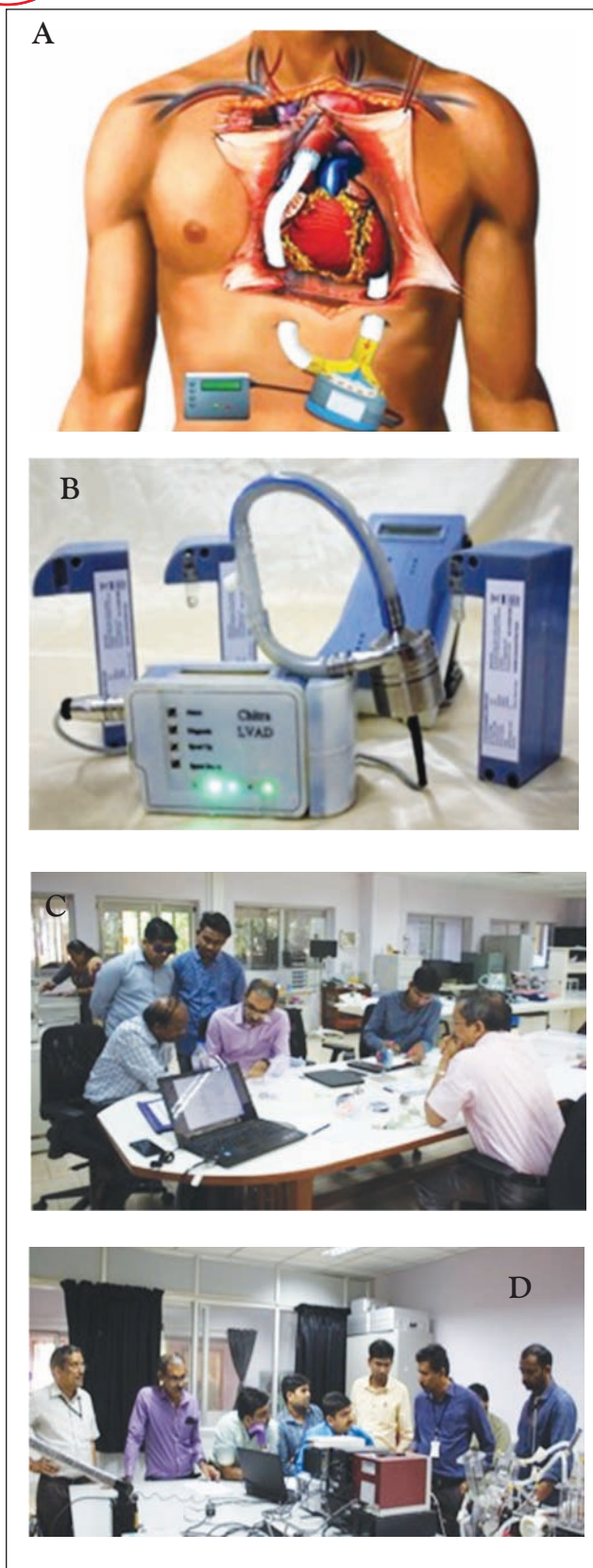
Figure 28. (A) Chitra paracorporeal Left Ventricular Assist Device (pLVAD), (B) pLVAD with controller, battery pack, and charging unit, (C,D) Training on device fabrication and evaluation to industrial partner (E,F) In vitro evaluation of LVAD for estimation of haemolysis
