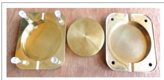
Brass electrodes for R F welding - weld, weld head and weld base
