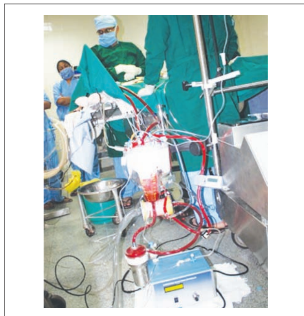
Figure 30. Chitra blood pump during ex-vivo animal evaluation
